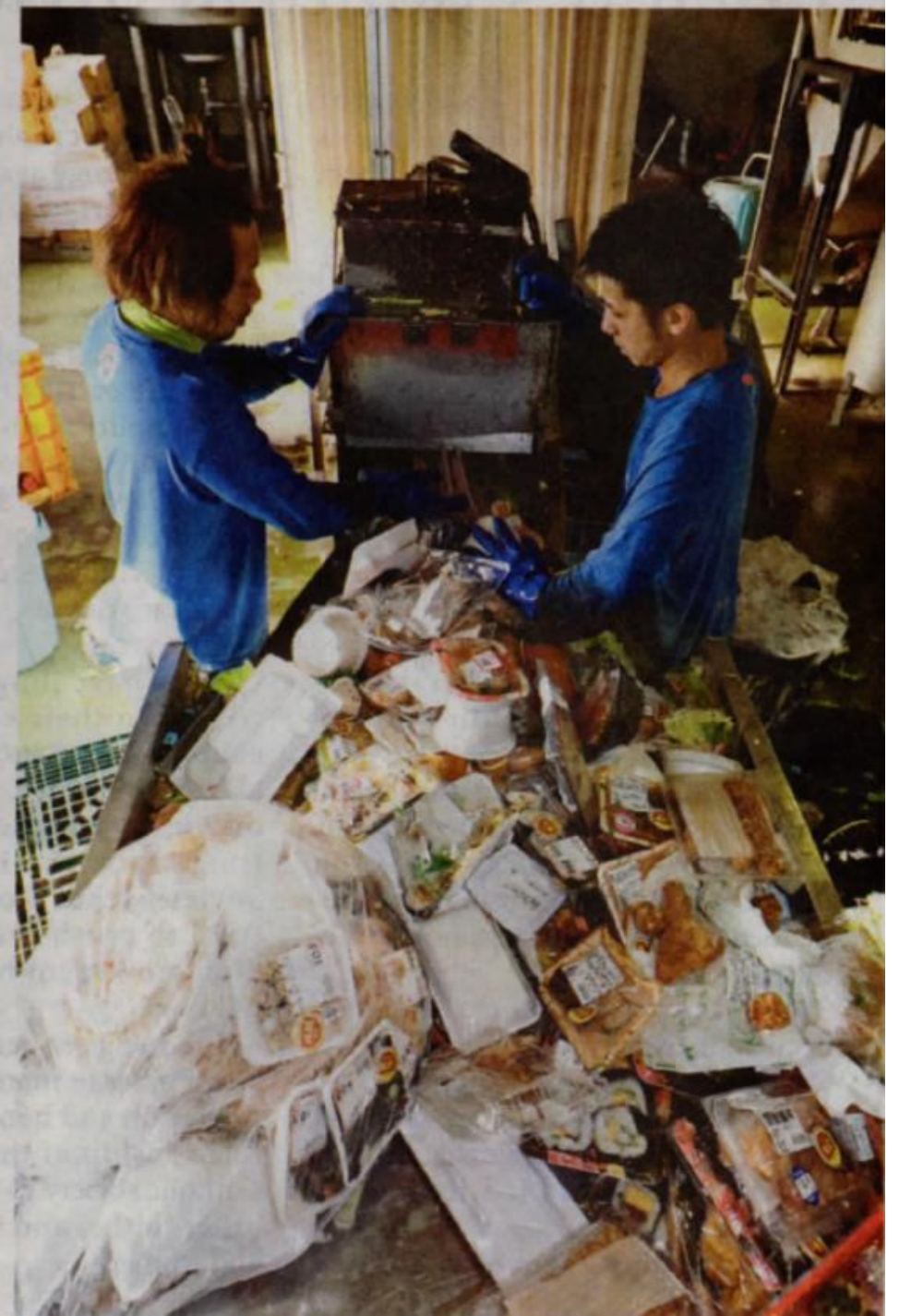
Workers guide leftovers from bento boxes and ready-made side dishes into a machine that separates food from wrapping in Nishi Ward, Fukuoka, on Dec. 14.
